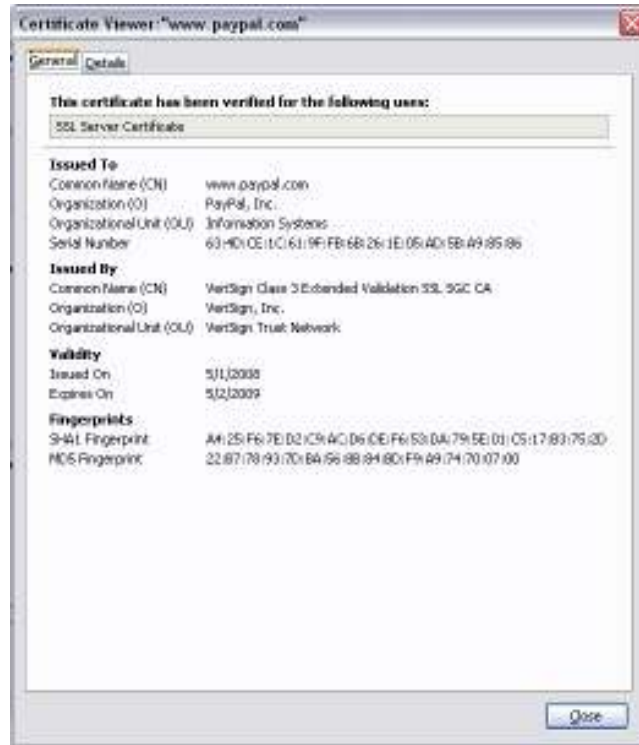
Figure 2 Digital certificate received from PayPal web server as viewed from a browser.
