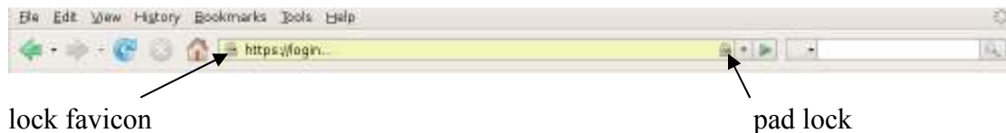
Figure 11 Positive feedback to the user by changing URL bar color and lock icons
