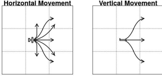
Figure 3: Grid-based vertical and horizontal aircraft movement model
